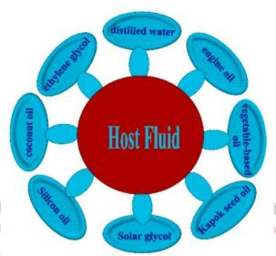
Figure 3 Some base fluids used as host medium of dispersed nanoparticles [5]
