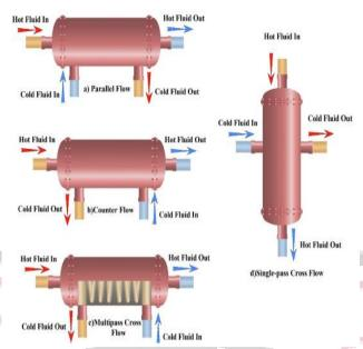
Figure 9 Type of flow in heat exchanger
