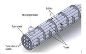
Figure 11 Baffles in Shell and Tube Heat Exchanger
