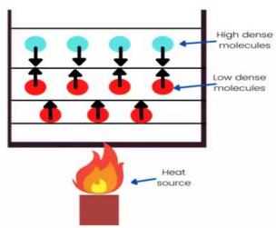
Figure 6 Free Convective Heat Transfer
