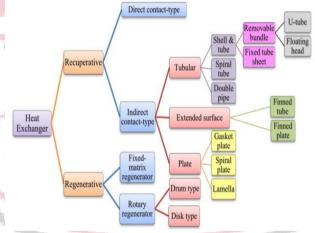
Figure 10 Classification of heat exchangers
